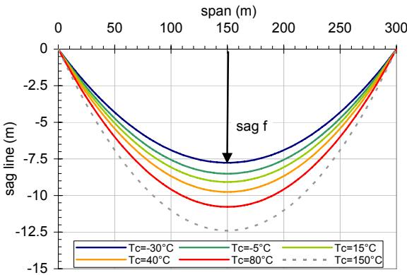
Fig. 5: Sag line depending on the conductor temperature, linear model according to standard
