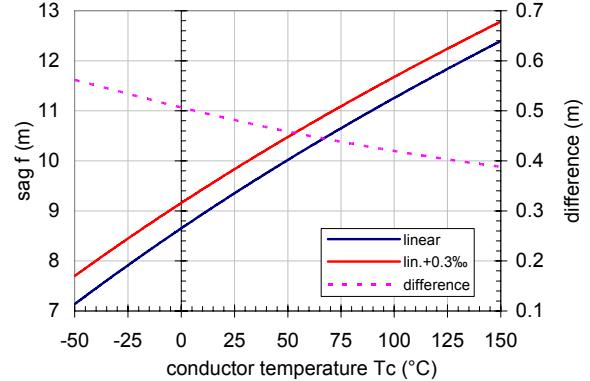
Fig. 6: Sag behaviour depending on the conductor temperature comparing a uniform composite and an aged linear model (additional elongation 0.3%)
