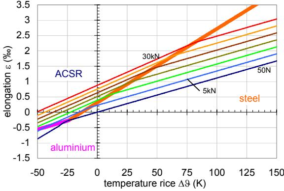
Fig. 4: Temperature elongation behaviour depending on mechanical force with 0.3% elongation of the aluminium wires
