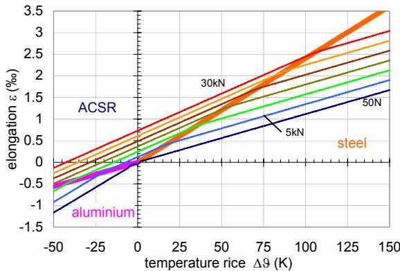
Fig. 2: Temperature elongation behaviour depending on mechanical force
