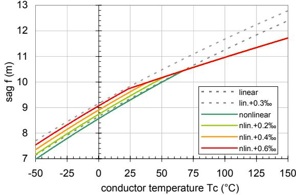
Fig. 8: Sag behaviour with different elongation of the aluminium wires depending on the conductor temperature
