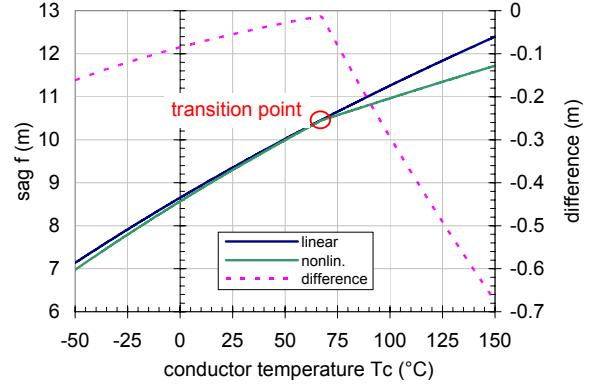
Fig. 7: Sag behaviour depending on the conductor temperature comparing a uniform composite and a nonlinear model
