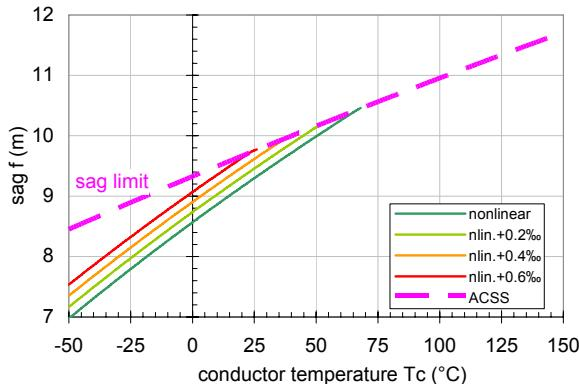
Fig. 9: Sag behaviour depending on the conductor temperature comparing with ACSS behaviour
