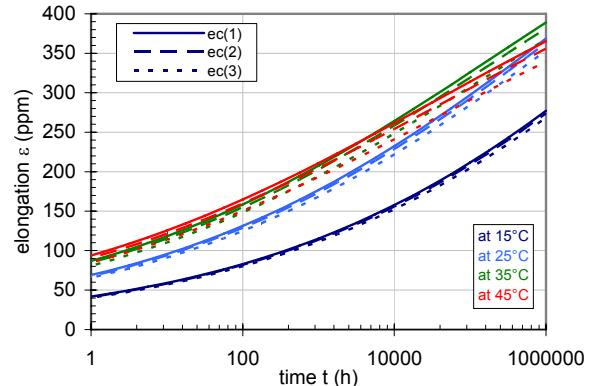
Fig. 3: Aluminium elongation of layers (1) ÷ (3) at 22kN force depending on the conductor temperature
