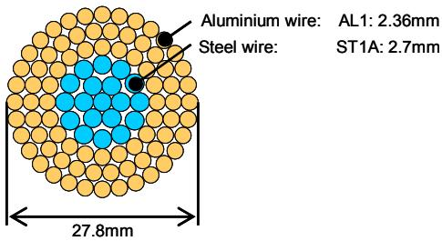
Fig. 1: Cross section of the 341-AL1/109-ST1A conductor
