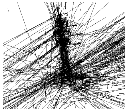
Figure 6. 3D line segment hypotheses before the grouping and outlier removal procedure. Our approach generates 71538 segments from 106 views. Note that there is a large number of outliers due to incorrect matches, but the power pylon which appears in the imagery is clearly recognizable.
