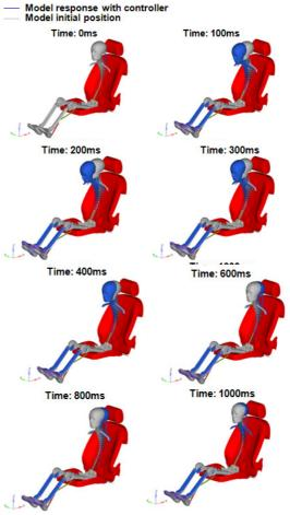
Figure 5. Model response to a 50 ms 4 g square pulse
