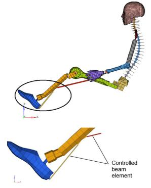
Figure 4. Model consisting of BIORID II and H3 dummy parts, detail muscle implementation
