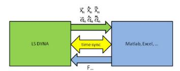
Figure 2. Coupling Exchange parameters
