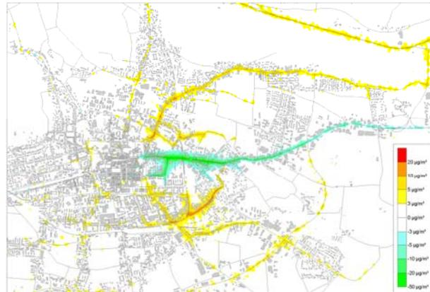
**Figure 12: Impact of the closure of one main street on the PM10 concentration (daily mean value)**
