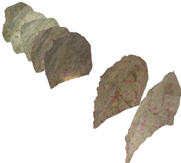
Figure 11: 3D images of a face successively arranged according to drift advance. The advance direction is from bottom-right to top-left. At the face images the rock mass structure, reference points and the bore hole pattern for the blasts can be observed. Note that the face of the third round has not been recorded.
