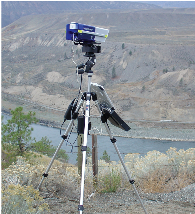
Figure 1: Panoramic line scanner with camera unit, motor, control notebook, power supply and tripod. Note that the scanner is several hundreds of metres apart from the imaging area. Images were taken during scanning a landslide near Ashcroft, BC, Canada.
