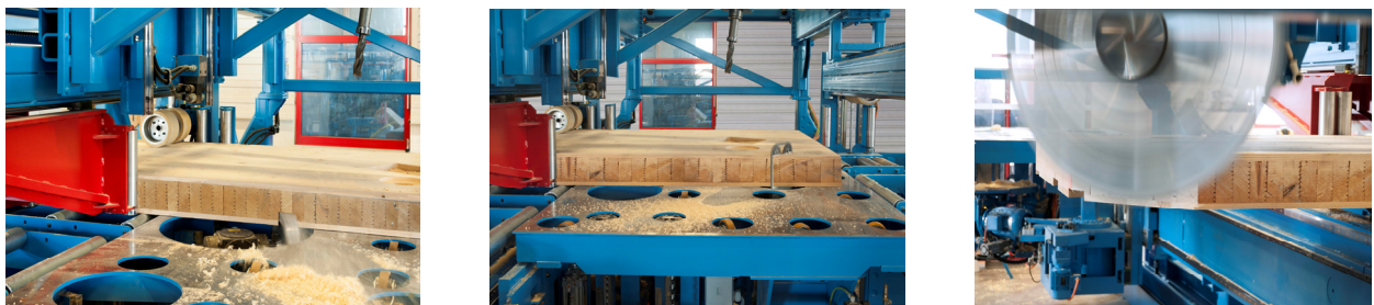
Fig. 9: Machining centre: moulder (left), chain saw (middle), saw (right) (© Hans Hundegger Maschinenbau GmbH / DE)
