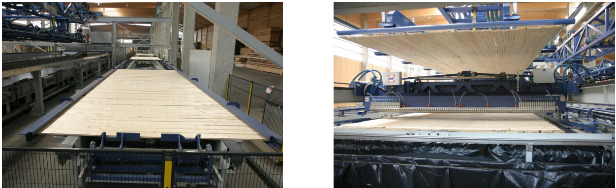
Fig. 6: Placing and aligning of the single layers (left); positioning of layers and application of adhesive (right) (© Minda-Industrieanlagen GmbH / DE)
