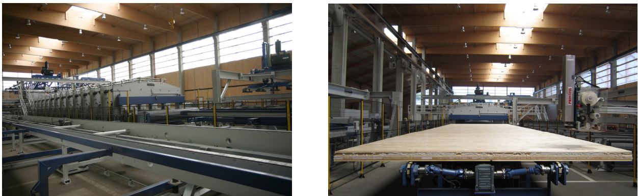
Fig. 7: Hydraulic surface and edge pressing device (left); unloading of ready produced CLT (right) (© Minda-Industrieanlagen GmbH / DE)
