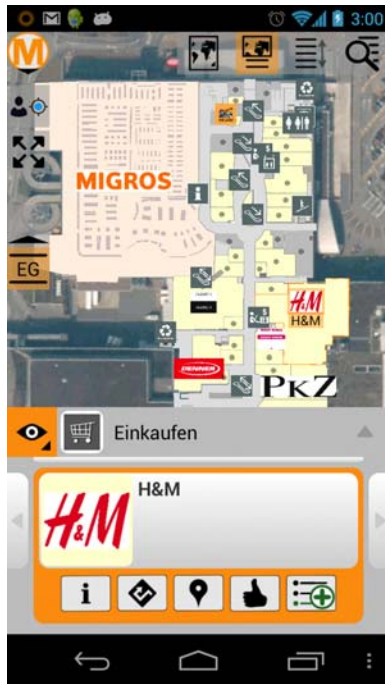
Figure 7 Split map/text user interface of the customer's location aware LBS shopping smartphone
