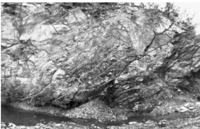
Figure 3: Image taken at a limestone quarry. The main geotechnical structures are annotated by an experienced geologist directly on the computer's screen. The resulting two-dimensional structural maps are displayed as graphical overlays and hierarchically managed.
