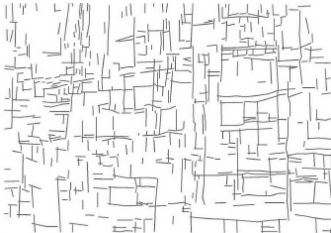
Figure 6: Discontinuity trace map. Horizontal discontinuity traces: bedding planes, 276 samples, vertical discontinuity traces: joint planes, 289 samples.
