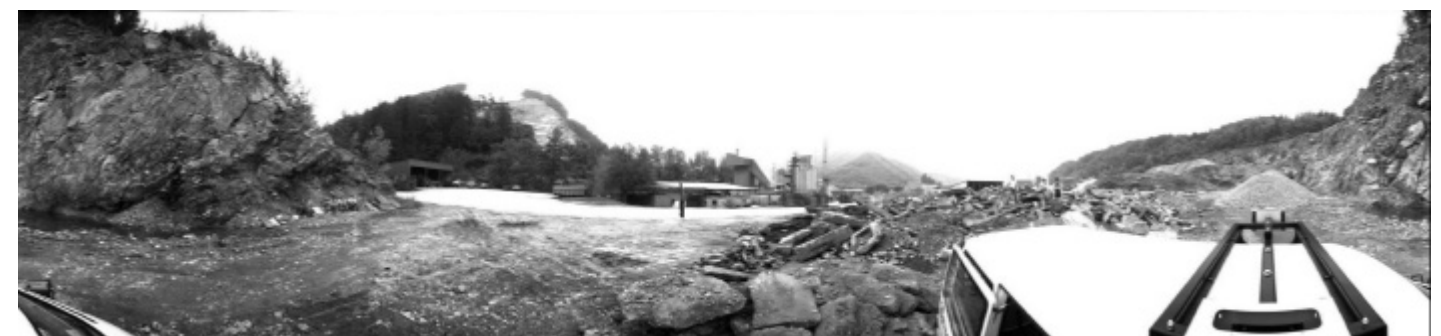
Figure 2: Panoramic image taken at a limestone quarry in Austria. The image shows a full 360 degree panoramic sweep and has a size of 27000x6000x3 pixels (uncompressed image: 460MB) at full resolution. The rock wall in the left is about 8 m high, but details in the sub-cm range can be identified.
