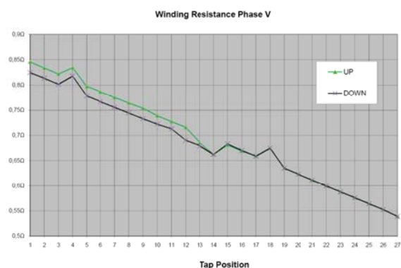
Figure 2: Example of a winding resistance test with the result of increased contact resistance [2]
