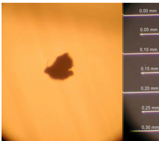
Fig. 2: Impurity of 55 \mu\text{m} in sample 1, impulse test level 480 kV
