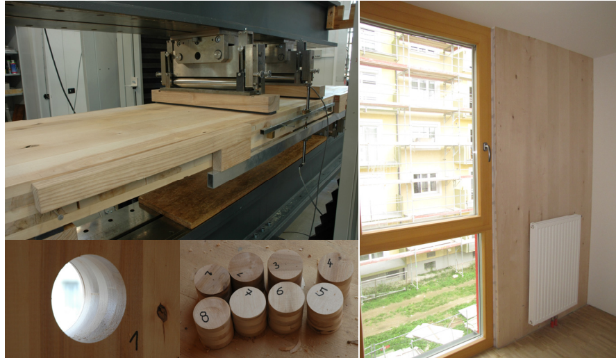
Fig. 4 test configuration for bending test birch-CLT (top left) [15] taking of core samples on the spot for delamination tests (down left) wall of birch-CLT – visual quality (right)
