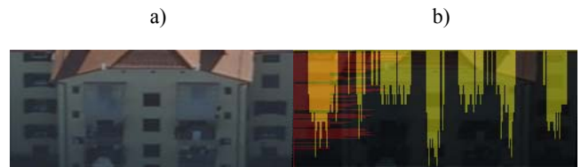
Figure 7: To the left is a rectified facade image with a depth structure, to the right a failed count of windows. The 3D structure needs to get considered.
