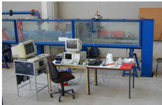
Figure 9: Test facilities for employing the UVP-Monitor in the study of open channel flow.
