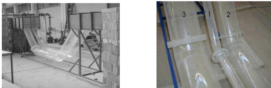
Figure 2: Test pipes, numbered 1 to 3. Overview (left) and close-up of elbows (right).
