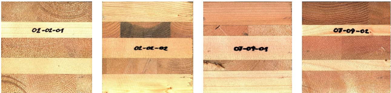
Figure 6: Pictures of some test specimens of industrially manufactured CLT [9]
