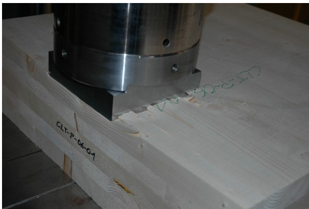
Figure 11: CLT plates with partly distributed loads – deformations [9]
