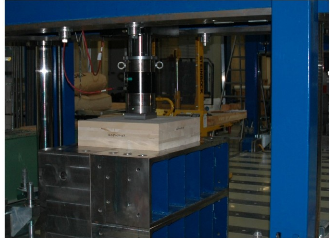
Figure 10: Test configuration and test arrangement for CLT with partly distributed loads [9]
