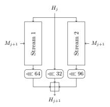
Fig. 1. Structure of the RIPEMD-128 compression function.
