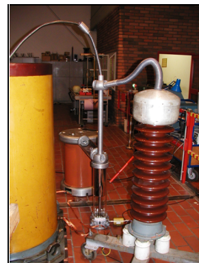
Fig. 7: Test setup in the laboratory - PD measurement according IEC 60270
