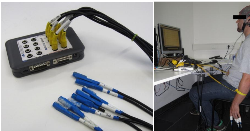
Figure 1. Left: Eight factors (blue) used for stimulation. The g.STIMbox is used to control the single factors and turn them on and off. Right: Setup of the experiment. Four factors are placed on the fingers of the left hand, the other four are placed on the fingers of the right hand. For electrical noise suppression in the EEG signal, the user is connected to ground (yellow stripe).
