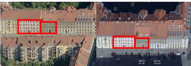
Figure 2: Oblique aerial image at 45° look angle taken from Microsoft Bing Maps (left); Vertical aerial image obtained from UltraCamX at a look angle of 27° (right).
