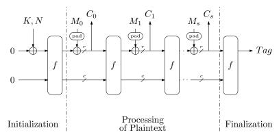
Fig. 1: Simplified sketch of LAKE KEYAK encryption (without associated data).
