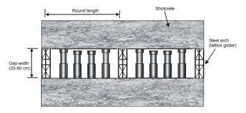
Fig 11. Typical assembly of LSC groups between steel arches
