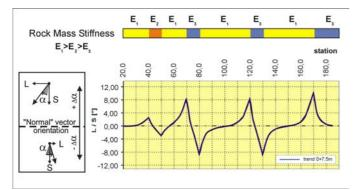
Fig. 4. Variation of displacement vector orientation when tunnelling in a heterogeneous rock mass, result of numerical simulation
