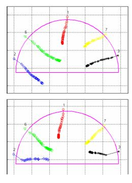
Fig. 2. Displacement vector plots of two measuring sections with a distance of 10 m, showing different behaviour
