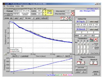
*Fig. 7.* Comparison between predicted and measured values at the Strenger tunnel.
