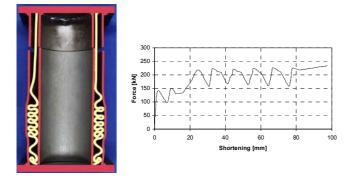
*Fig. 10. Yielding element after laboratory testing (left), and load line (right)*
