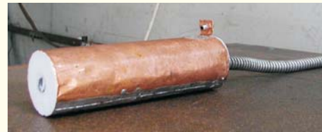
Cable model with open-cell foam as insulation medium (left) and test vessel
