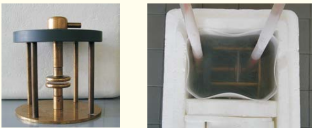
Test electrodes (left) and test vessel (right) for electric breakdown tests
