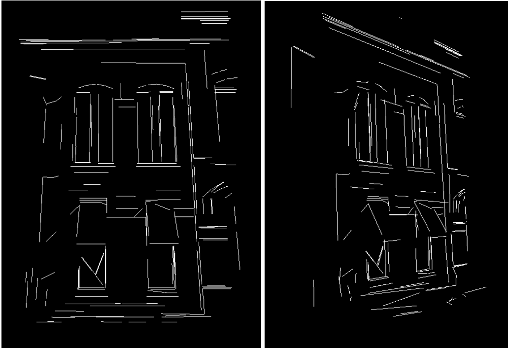
Figure 7: Vectors extracted from the overlapping terrestrial photographs in Figure 6. These 3-d vectors have been computed automatically and can now be submitted to a machine-supported manual editing and clean-up procedure.
