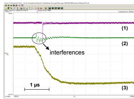
Fig. 9: Comparison of PD impulse in air - optical (1) and wide band conventional (2) system during negative impulse voltage (3).
