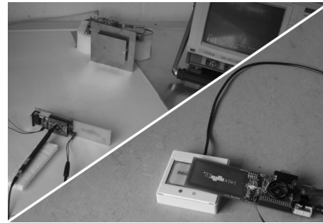
Fig. 3. Picture of the measurement setup using UHF (upper left) and HF (lower right) RFID-tag prototypes.
