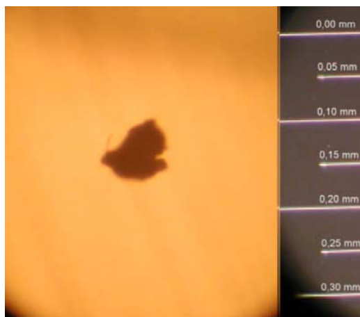
Fig. 2: Impurity of 55 \mu\text{m} in sample 1, impulse test level 480 kV
