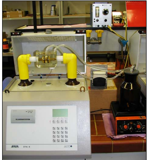
Picture 9: Integration of the new oil test cell in a standard oil breakdown test device
