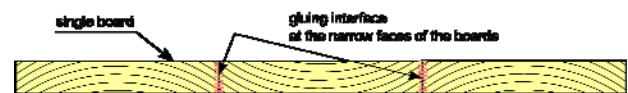
Figure 4: Single layer of a RVE element with lateral gluing interfaces at the narrow faces
