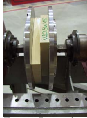
Figure 20: Test specimen for torsional shear strength
