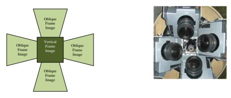
Figure 2: The Maltese Cross configuration with five camera heads (left) and an realization in the form of the TrackAir Midas System (right). Source: Petrie (2008)
