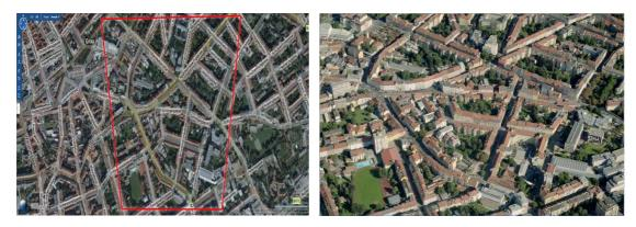
Figure 3: Detail from Microsoft Bing Maps. Left is the orthophoto and superimposed the outline of an oblique aerial image produced with the Pictometry system operated by Blom. Right is the oblique aerial image.
