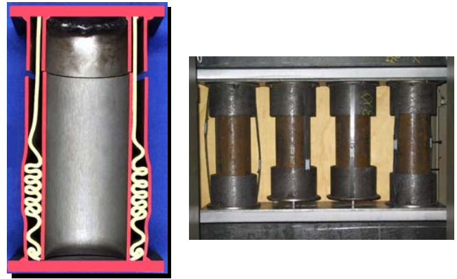
Figure 4. Left: section through improved yielding element with concentrically arranged steel tubes [10]; right: group of 4 elements assembled for the installation in the lining
