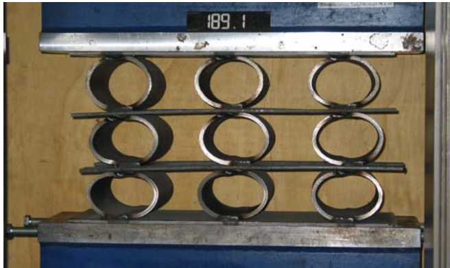
Figure 6. Yielding steel element, as produced by Bochumer Eisenhütte (BE)
