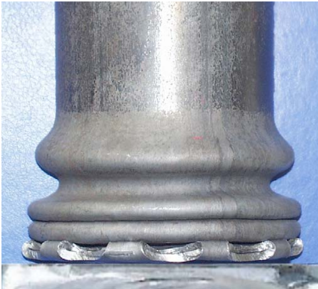
Figure 3. Buckling of steel tube in the laboratory test. Foto: Schubert
