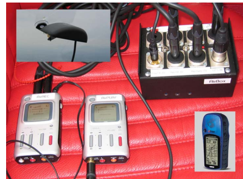
Fig. 2. Complete voice channel measurement system on-board an aircraft, with audio player and recorder, interface box, synchronisation GPS (top left), and tracking GPS (bottom right).
