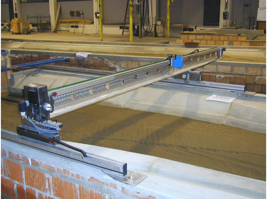
Figure 5: Measurement setup for river bed mapping at Hermann-Grengg Laboratories.
