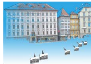
Figure 9: MetropoGIS uses a fully automated approach to create 3D models of urban spaces using a limited number of images. This example is of Graz Hauptplatz.
