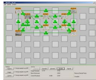
Figure 5: Graph showing the images taken for a particular scene, and the relationships between those images (overlaps, orientations).
