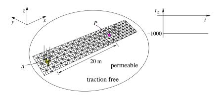
Figure 1: Half space under vertical load: Discretization and load history
