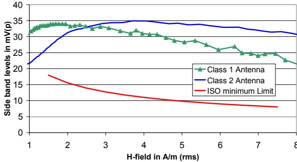
Figure 7. Load modulation measured for SmartCards with full size (class 1) and half-size (class 2) antenna and chips with described properties.
