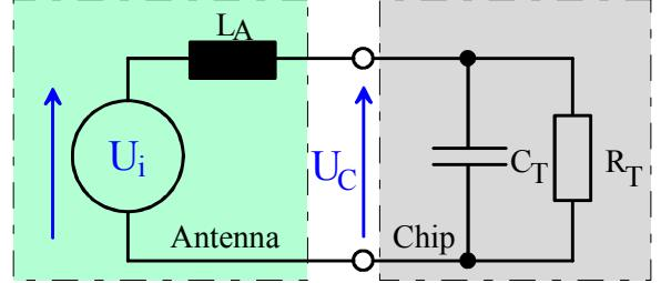
Figure 5. Equivalent Transponder circuit for energy considerations.
