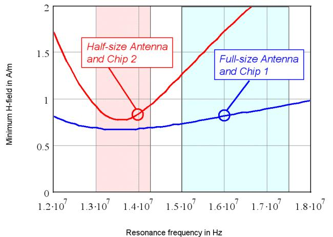
Figure 6. Minimum H-field required for operation.
