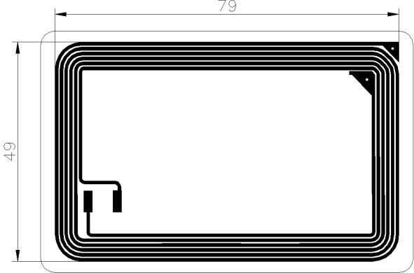
Figure 3. Full size (class 1) etched antenna layout.
