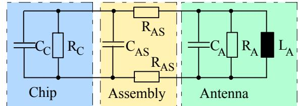
Figure 2. Contactless SmartCard electrical system equivalent circuit.
