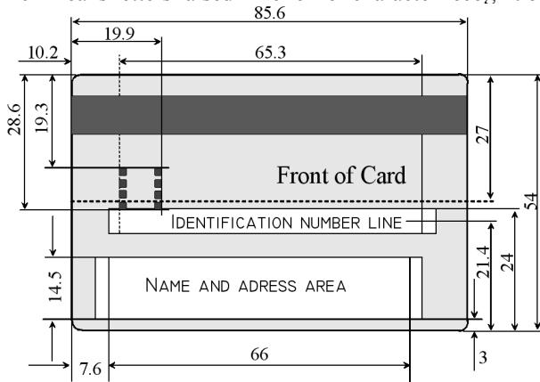
Figure 1. Card geometry specifications in millimeters.
