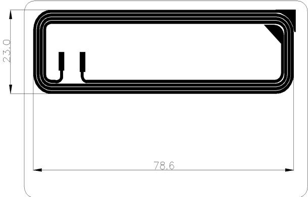
Figure 4. Half size (class 2) etched antenna layout.
