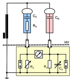
Fig. 1: Capacitance and Dissipation Factor Bridge (Schering Bridge) [2]
