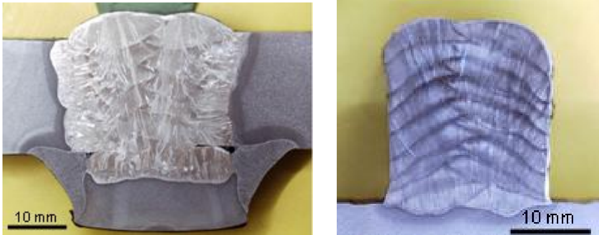
Fig. 13: all weld metal test specimens: left: all weld metal acc. EN 1579-1 (AWM); right: plate deposit (PD) [7]
