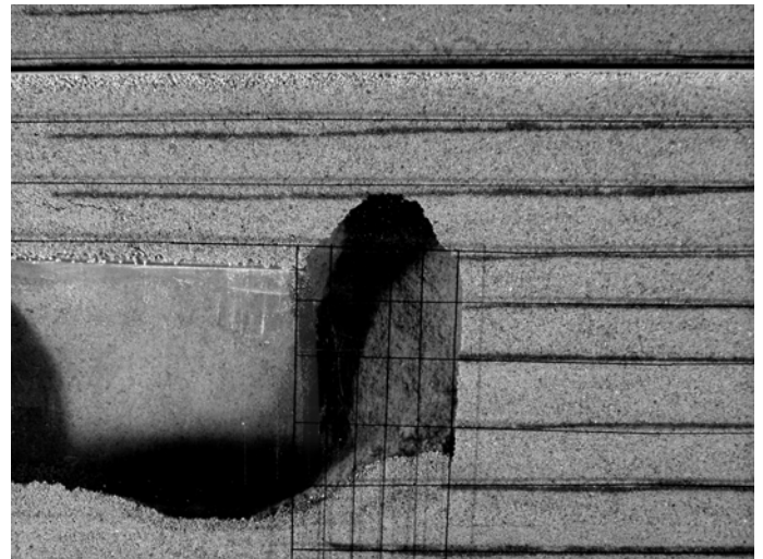
Figure 1. Typical overbreak at unsupported span in model test
