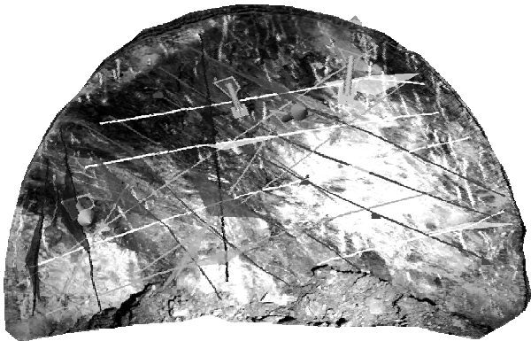
Figure 1: Evaluated 3D image showing discontinuity traces and areas with corresponding orientations.
