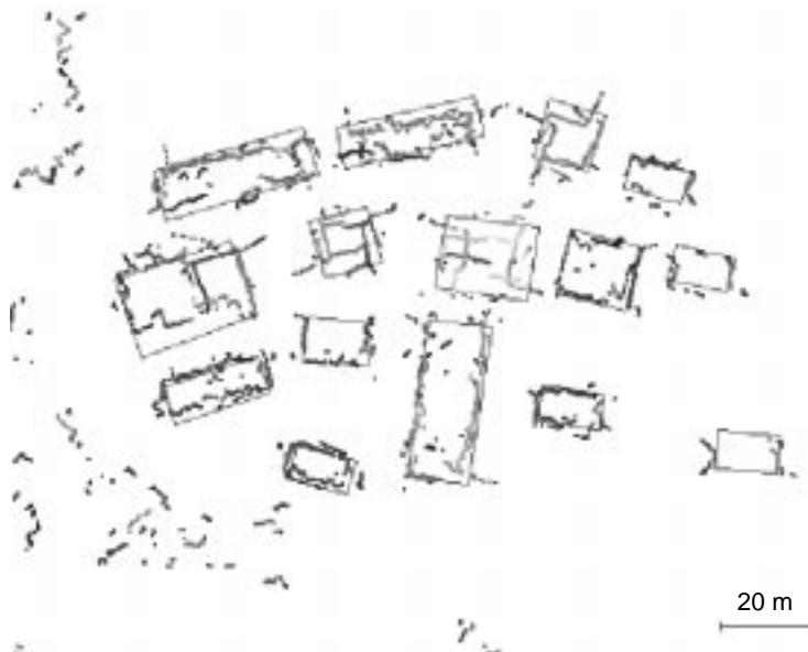
Figure 6: Reconstructed building walls of the whole building ensemble on the MOUT testsite with overlaid building outlines from ground truth data.
