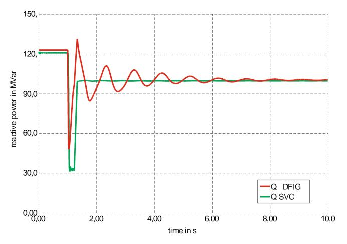
case with reduced fault clearing time
