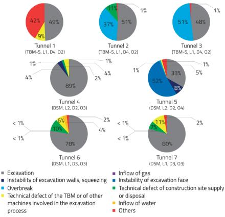
Figure 3. Evaluation of the unexpected standstills of seven projects (maintenance shifts: for Tunnel 1-3 included in "Others"; for Tunnel 4-7 included in "Excavation").
