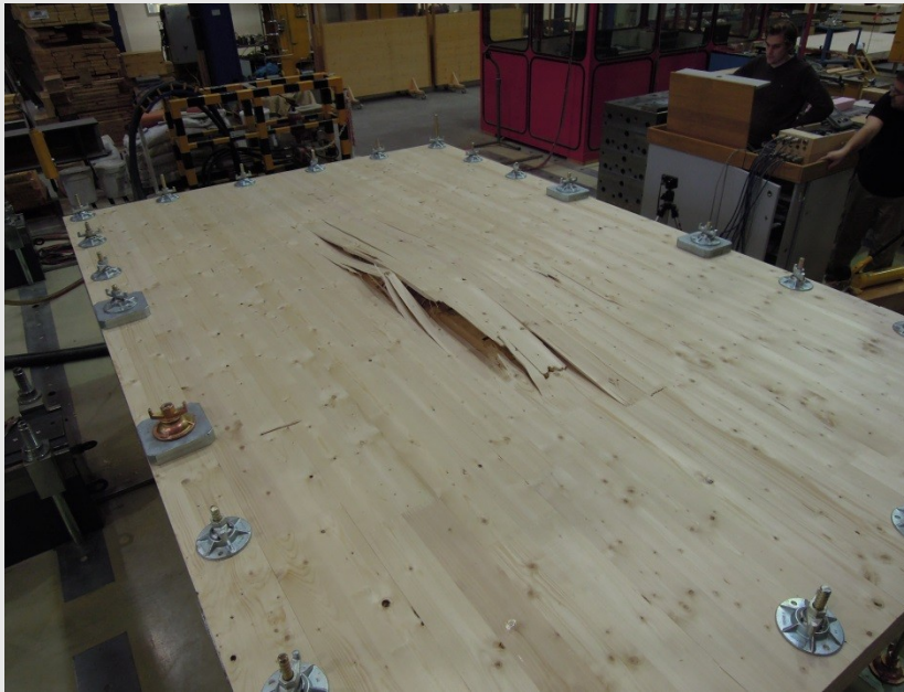
failure of CLT 7s
