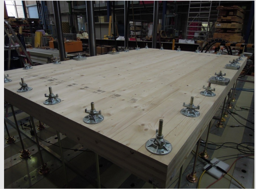
7-layered, biaxial loaded CLT ( CLT 7s )
