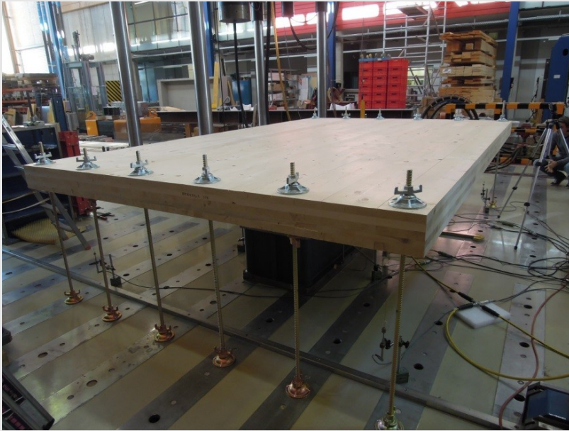
5-layered, uniaxial loaded CLT ( CLT 5s )
