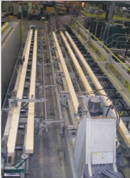
Test site/arrangement for experimental investigation of length effect of brittle materials (2005-07)
