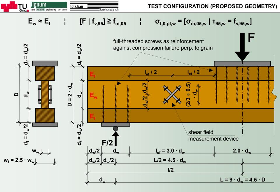
ISO/FDIS 8375:2008 (prismatic) I<sub>ef</sub> ≥ 2.0 · D | Schickhofer (2001; I-beam) I<sub>ef</sub> = 3.3 · d<sub>w</sub>; L = 5 · D
