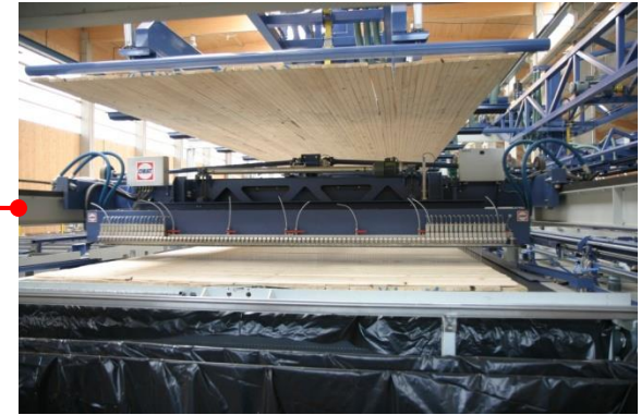
adhesive application next layer stand-by
