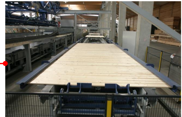
cross layers composing & compressing
