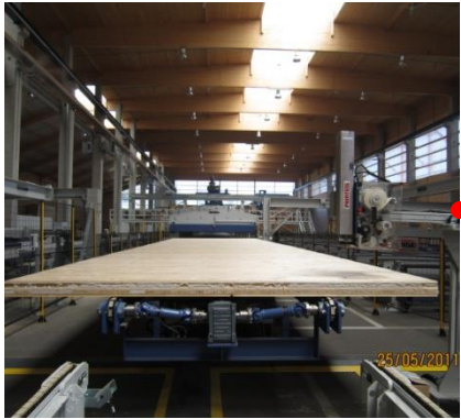
CLT element ready for cutting and joining
