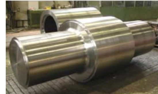
Turbinen Rotor (COST FB2)
