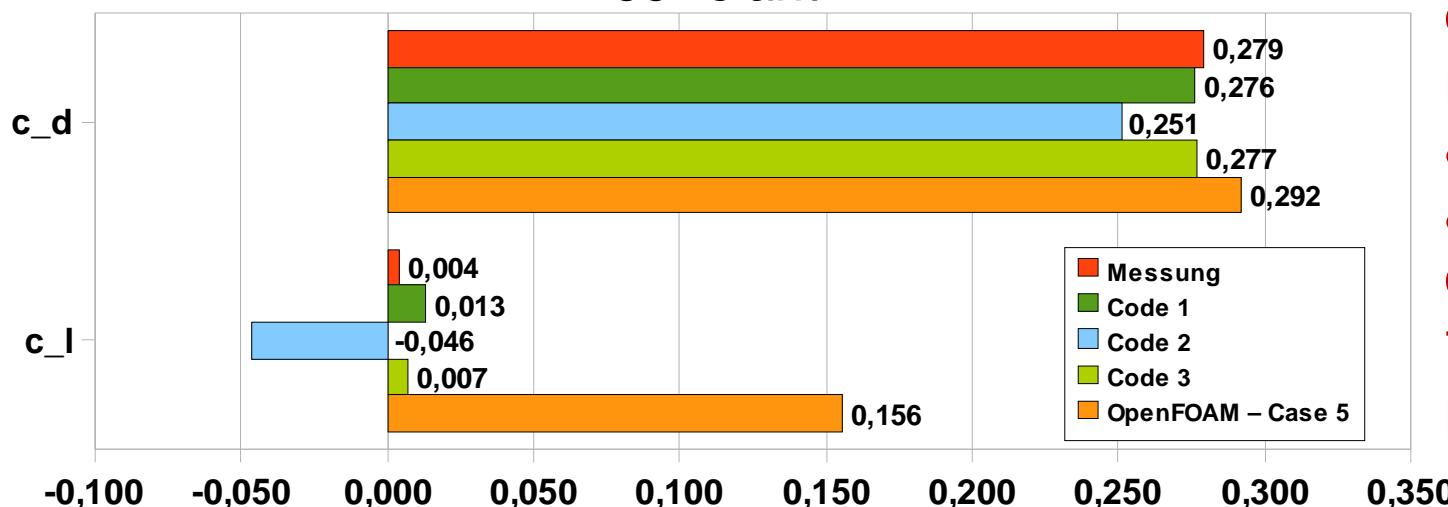
Strong deviation of lift coefficients from measurement data in all cases with 35° slant; apart from this, quality of results is similar to the results from other programs
