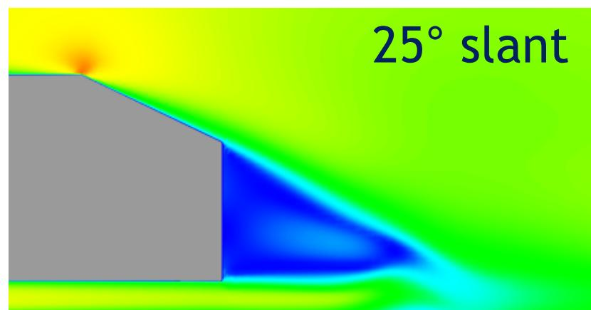
➡ Attached flow over the slant
