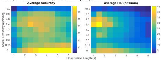
Figure 1. Average SSVEP accuracy and ITR of the four-class SSVEP BCI from experiement 1. The accuracies and ITRs are shown for the nine different spatial-frequency conditions as well as for varying time-window lengths used in the CCA based classification.
