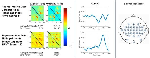
Representative data of a subject with CP and typically developing counter part. Left: Heat map of funcitonal connectivity based Figure 1. on electrode connectivity. Center: Grand average P300 of Pz electrode. Right: Electrode montage used.
