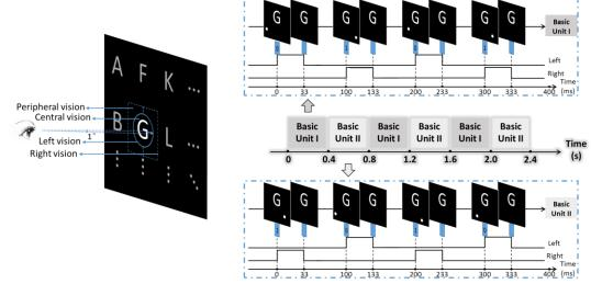
*Figure 1.* (Left) Central, peripheral, left and right visions of the target character defined in this study. (Right) Timing sequence of a completed trial for letter 'G' are displayed with the discription of the two basic units.
