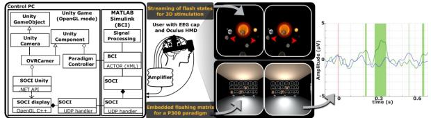
*Figure 1.* Architecture of the SOCI Unity plugin (left) and stereoscopic view of two demo applications using a c-VEP (center, right) and P300 paradigm (center, bottom). On the right side the mean target (green line) P300 over Cz of S2 after 90 trials is plotted, while the green area indicates significant (p<0.05) deviation compared to a non-target average P300.
