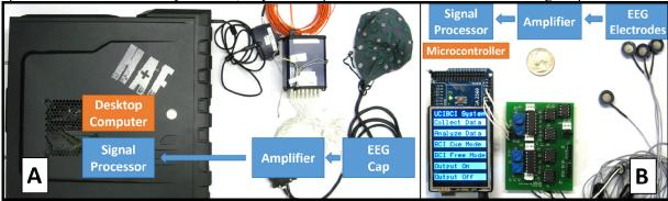
*Figure 1. A*: A traditional BCI system (~\$30,000). **B**: The developed, miniaturized BCI system (~\$300). In both systems, brain signals are captured by the EEG cap/electrodes, amplified, and then sent to a processor for decoding.
