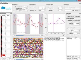
*Figure 1.* User interface of Turbo-Satori. The user is able to inspect channels in detail and combine them in one view. All preprocessing parameters can be adjusted in on-line and are accessable during data acquisation. A log window shows current information.
