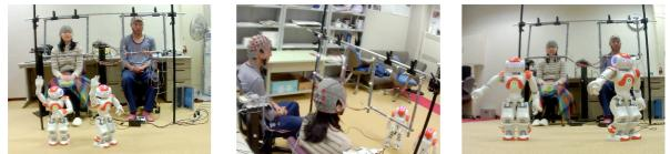
Figure 1. Three screenshots from a video available online [3] documenting the succesful synchronized control of two robots using eight commands' cVEP BCI scenario.
