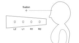
Figure 1. Schematic of visual perceptual light stimuli. The fixation LED was positioned 5 cm above the center of the stimuli. Four visual targets were at 60cm viewing distance and were at 2.5 and 7.5 degree visual angle to the left and right of body midline / straight ahead.
