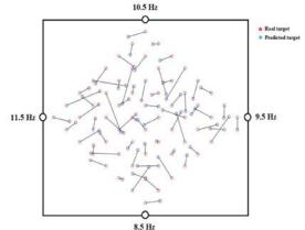
Fig 1. LEDs position and errors for the best performing subject. Each segment represents the distance between the real (red) and estimated (blue) target.
