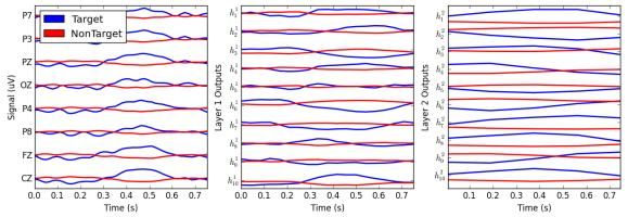
Figure 1. Left) The mean target vs non-target signal values for each channel. Center) The mean response for each hidden unit in the first convolutional layer. Right) The mean response for each hidden unit in the second convolutional layer.
