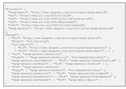
Figure 10: Security policy for service provided in JSON-LD format, excerpt
