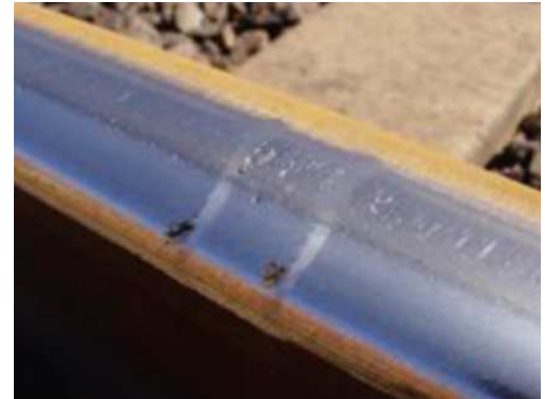
Localized spalling damage at FBW in hypereutectoid rail. source: [7]
