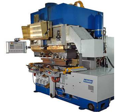
Schlatter GAA100 stationary FBW machine for rails. source: [8]
