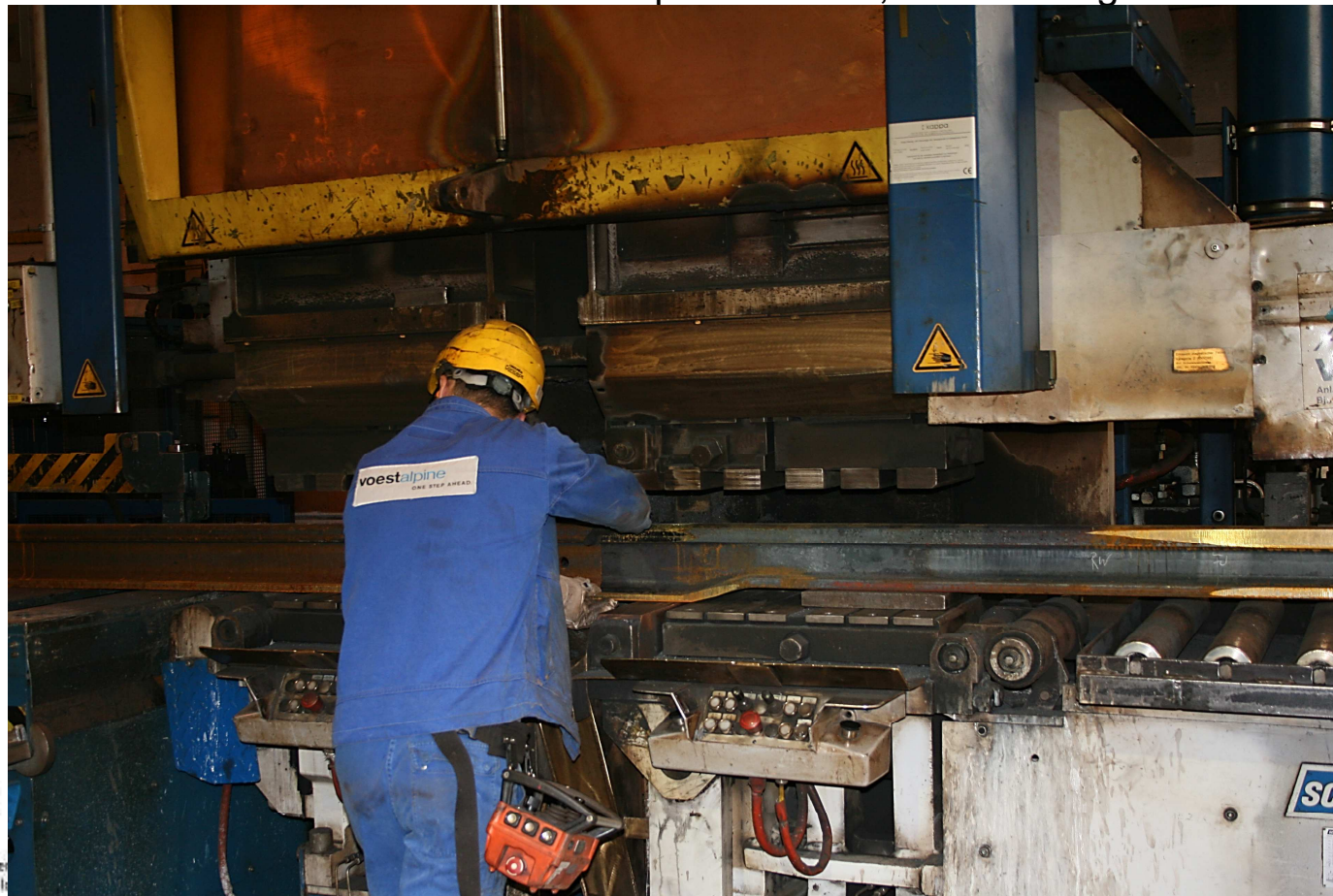
Schlatter GAA100 stationary FBW machine for rails. source: [8]
