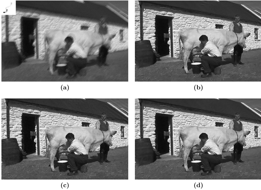
Figure 2.12: Deconvolution results of a random image sample from the BSD500 test set. (a) blurry observation with true blur kernel in upper left corner. Deconvolution results (b) IAM-DC 20 5×5 , (c) I 2 AM-DC 20 3×3 and (d) I 2 AM-DC 20 5×5 .
